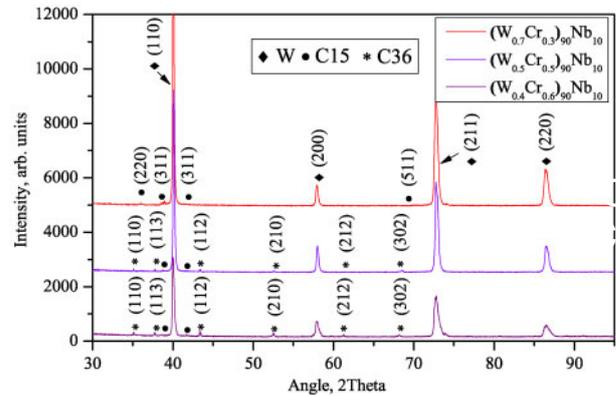
**3 X-ray diffraction patterns ( $Cu K_\alpha$  radiation) obtained from W–Cr–Nb alloys sintered at  $1790^\circ C$  for 5 h**
