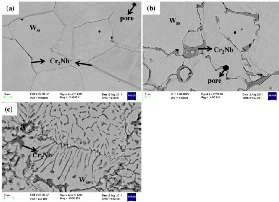
4 Images (SEM) (backscattered electron) of *a*  $(W_{0.7}Cr_{0.3})_{90}Nb_{10}$ , *b*  $(W_{0.5}Cr_{0.5})_{90}Nb_{10}$  and *c*  $(W_{0.4}Cr_{0.6})_{90}Nb_{10}$  alloys sintered at 1790°C for 5 h
