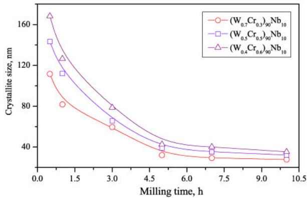
**2 Plots showing variations of crystal size of  $W_{ss}$  in W–Cr–Nb elemental blends with milling time up to 10 h**
