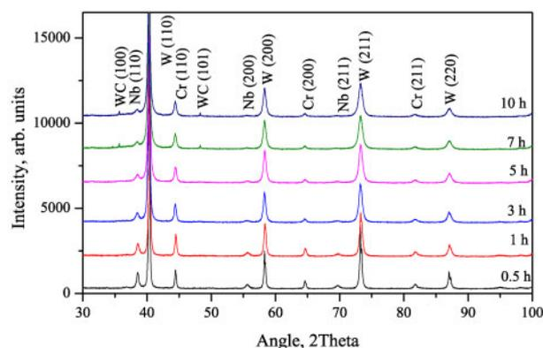
1 X-ray diffraction patterns ( $\text{Cu K}\alpha$  radiation) of  $(\text{W}_{0.5}\text{Cr}_{0.5})_{90}\text{Nb}_{10}$  elemental powder blend after milling for different durations
