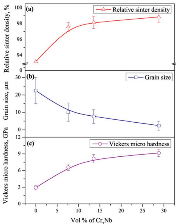
7 Relative sinter density, grain size and hardness of pure W and investigated W–Cr–Nb alloys
