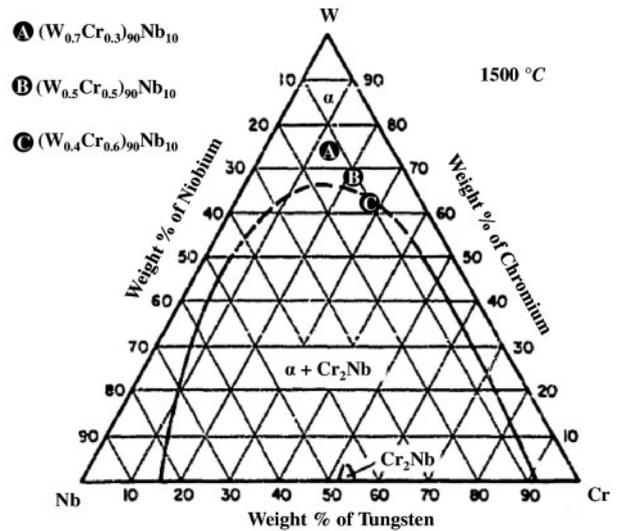
6 Isothermal section of W–Cr–Nb alloy phase diagram at 1500°C<sup>20</sup>
