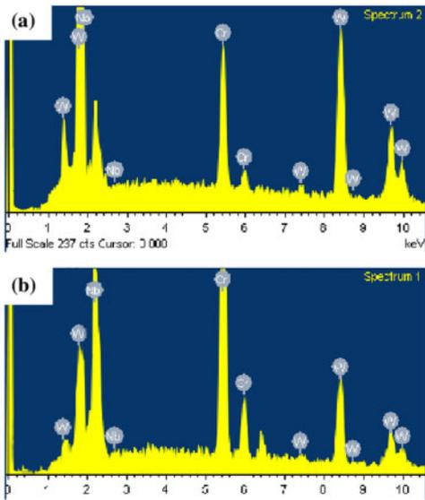
5 Energy dispersive spectroscopy spectrum from *a* brighter and *b* darker regions in microstructures of  $(W_{0.5}Cr_{0.5})_{90}Nb_{10}$  alloy
