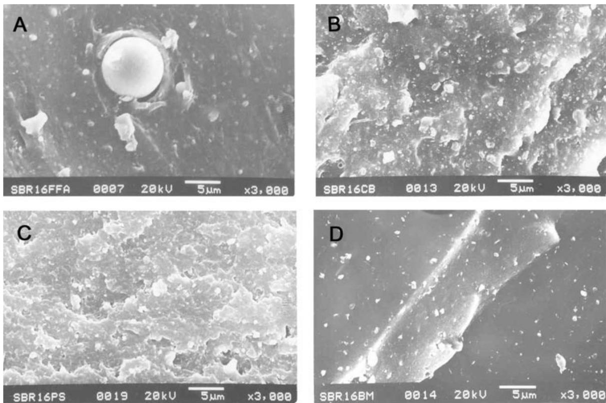
FIG. 13. SEM images of SBR composite with various filler at a dosage of 16 phr. (A) FFA-SBR composite at 3,000 times magnification, (B) CB-SBR composites at 3,000 times magnification, (C) PS-SBR composites at 3,000 times magnification, and (D) NFA-SBR composites at 3,000 times magnification.
