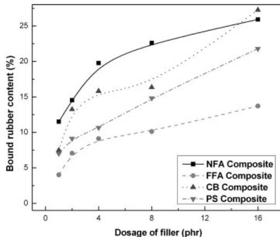
FIG. 12. Variation of bound rubber content with filler dosage.
