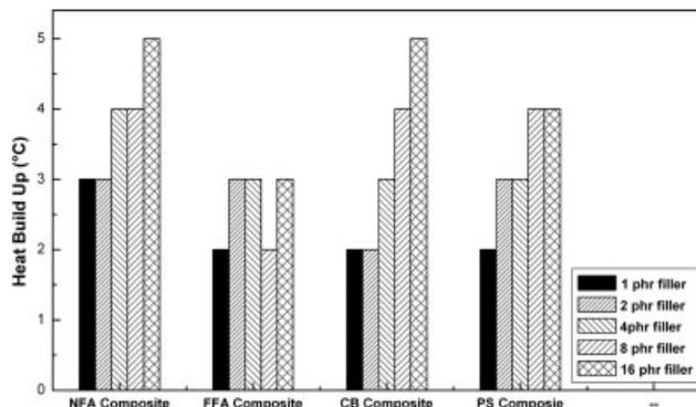
FIG. 8. Variation of heat build up with filler dosage.
