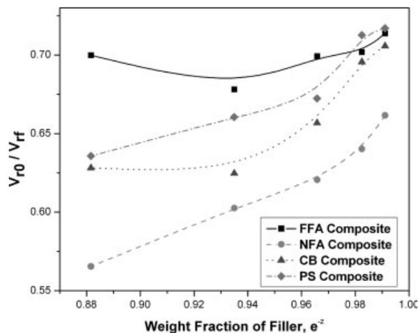
FIG. 10. Plots according to Cunen–Russel equation for composites for various fillers.
