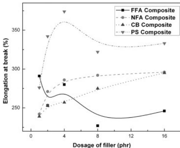
FIG. 3. Variation of elongation at break with filler dosage.
