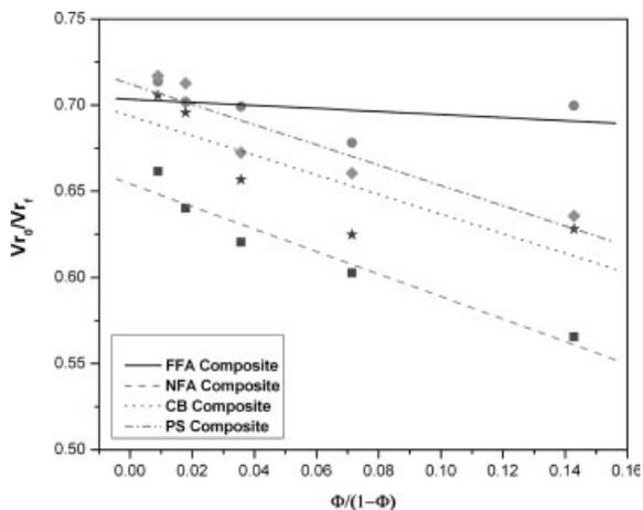
FIG. 11. Kraus' plot for various composites with various fillers.
