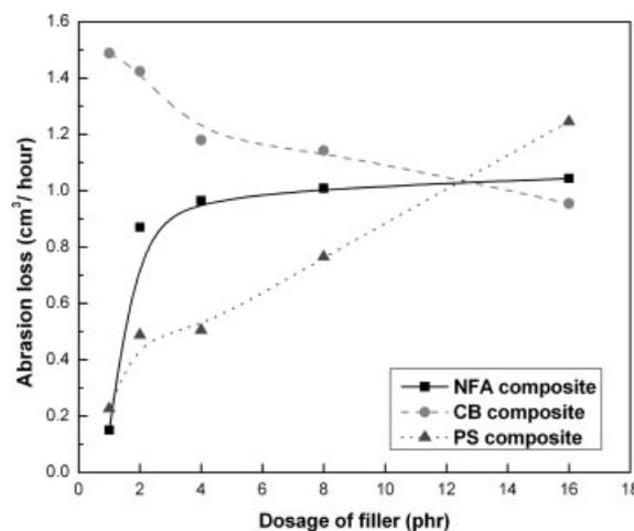
FIG. 5. Variation of abrasion loss with filler dosage.
