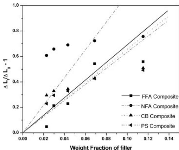
FIG. 1. Plots according to Westlinning–Wolff equation for composites with various fillers.
