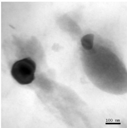
FIG. 14. TEM image of nanostructured fly-ash filled SBR composite.
