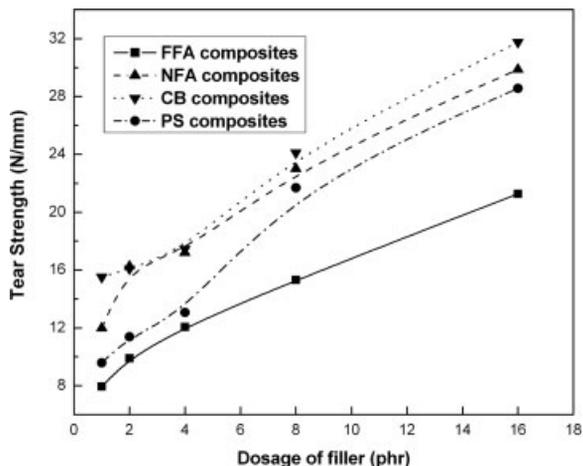
FIG. 6. Variation of tear strength with filler dosage.
