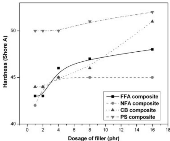
FIG. 7. Variation of hardness with filler dosage.
