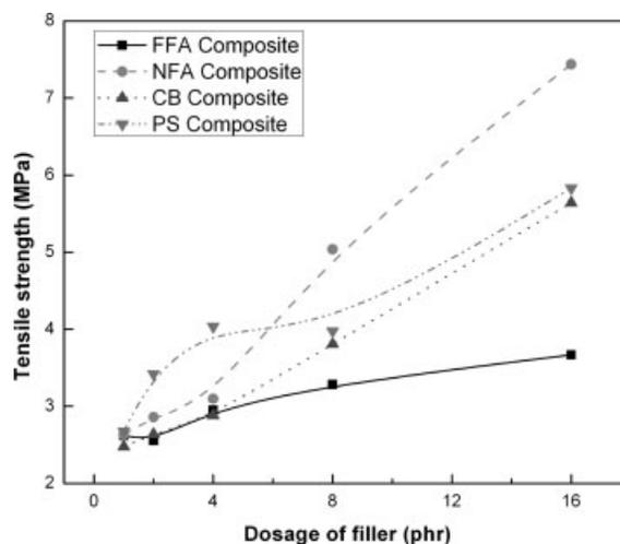
FIG. 2. Variation of tensile strength with filler dosage.
