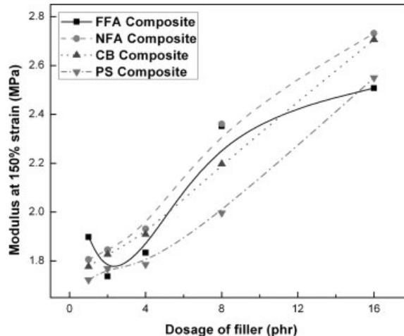
FIG. 4. Variation of modulus at 150% with filler dosage.
