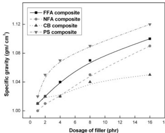
FIG. 9. Variation of specific gravity with filler dosage.
