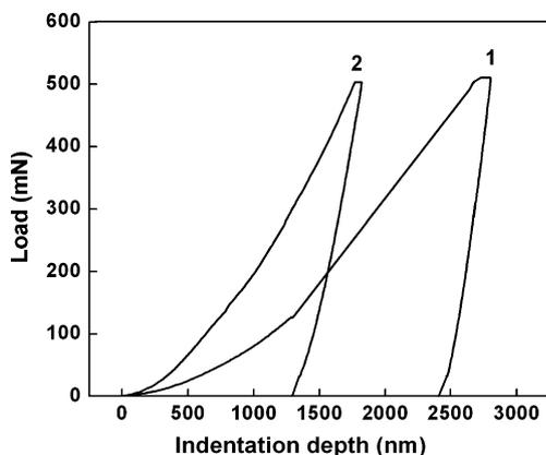
Figure 3. Load–displacement curves of as-received (plot 1) and laser surface nitrided (plot 2) (lased with a power of 800 W at a gas flow rate of  $101 \text{ min}^{-1}$ ) Ti–6Al–4V indented to a maximum load of 500 mN.
