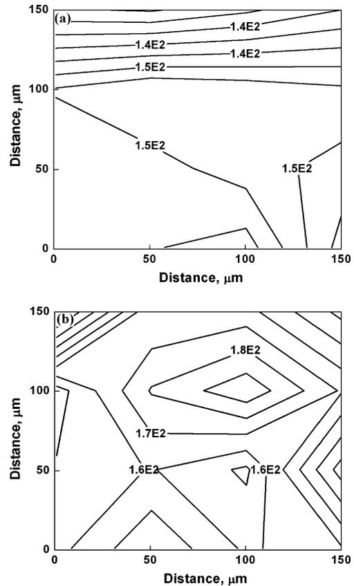
Figure 4. Iso-Young's modulus contour (in GPA) obtained from nanoindentation of (a) as-received and (b) laser surface nitrided (lased with a power of 800 W at a gas flow rate of  $101 \text{ min}^{-1}$ ) Ti–6Al–4V indented to a maximum load of 500 mN.
