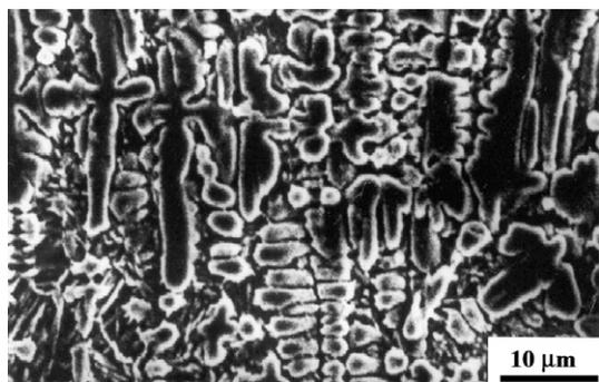
**Figure 1.** Scanning electron micrograph of the top surface of laser surface nitrided Ti–6Al–4V lased with a power of 800 W and gas flow rate of  $10 \text{ l min}^{-1}$ .
