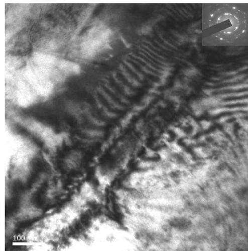
**Figure 2.** Transmission electron micrograph of the top surface of laser surface nitrided Ti–6Al–4V lased with a power of 800 W and gas flow rate of  $10 \text{ l min}^{-1}$ .
