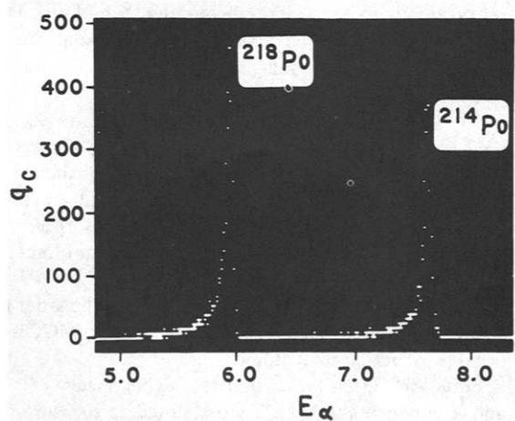
Fig. 4. A typical  $\alpha$ -decay spectrum recorded. Here  $q_c$  is the cumulative number of counts per channel per cycle of 1000 s, and  $E_\alpha$  is the energy of  $\alpha$ -emission in MeV.
