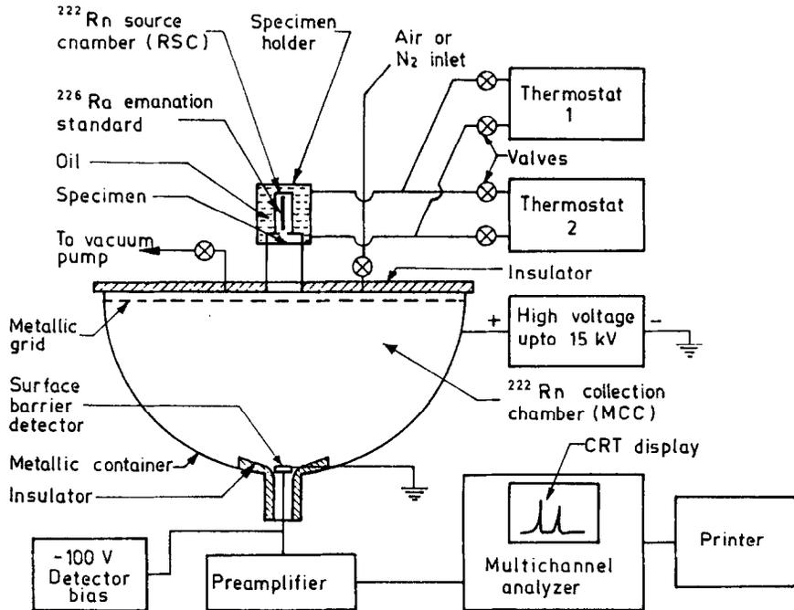
Fig. 2. Schematic illustration of the  $^{222}\text{Rn}$  diffusion measuring method.
