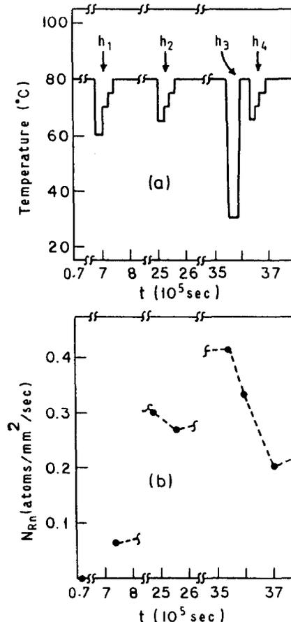
Fig. 6. (a) Thermal schedule of the foil specimen, (b)  $N_{\text{Rn}}$  measured at 80°C at various instances of this schedule. The discontinuity in time-scale is apparent in the plot.
