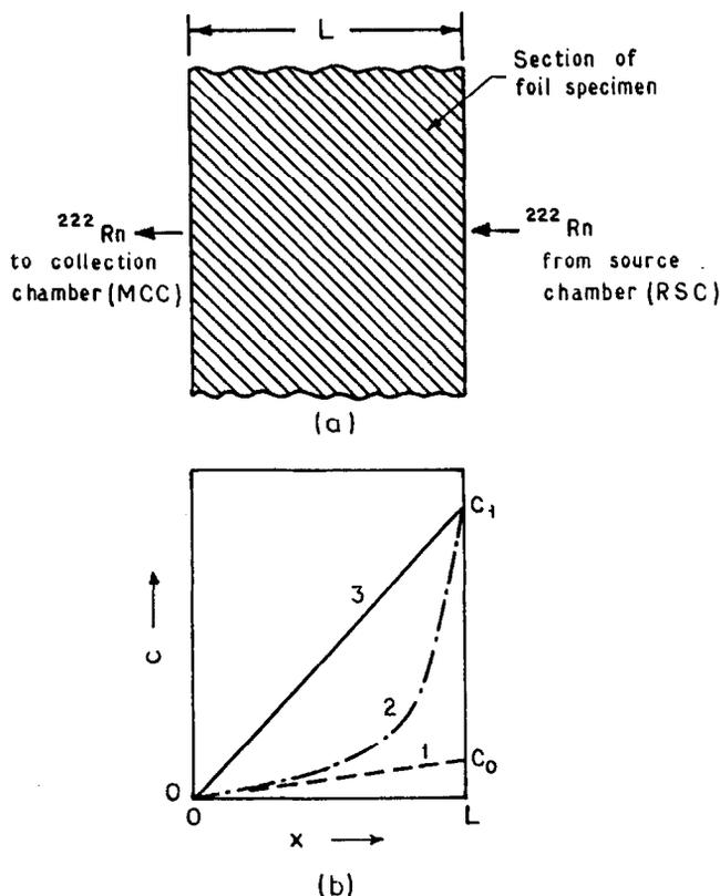
Fig. 3. (b) Schematic view of the variation of  $^{222}\text{Rn}$  concentration across the foil section displayed in (a). Curves 1 and 3 represent the steady-state concentration profiles at  $T_0$  and  $T_1$ , respectively. Curve 2 corresponds to a non-steady state following up-quenching from  $T_0$  to  $T_1$ .
