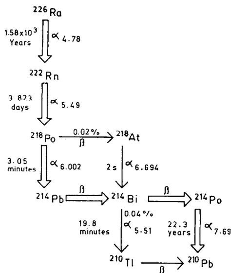
Fig. 1. The sequence of spontaneous nuclear decay of  $^{226}\text{Ra}$  along with the half-life of each component [3, 4]. The hollow arrows indicate the main reaction path and the thin arrows illustrate the secondary route taken up by a small percentage (indicated) of atoms.  $\alpha$  and  $\beta$  refer to the type of decay and the subscript of  $\alpha$  represents the maximum energy of this decay in MeV.
