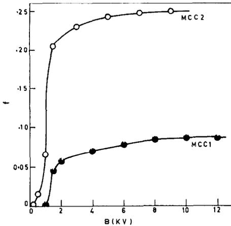
Fig. 5. Variation of the net collection efficiency  $f$  with the applied positive bias of the MCC walls.
