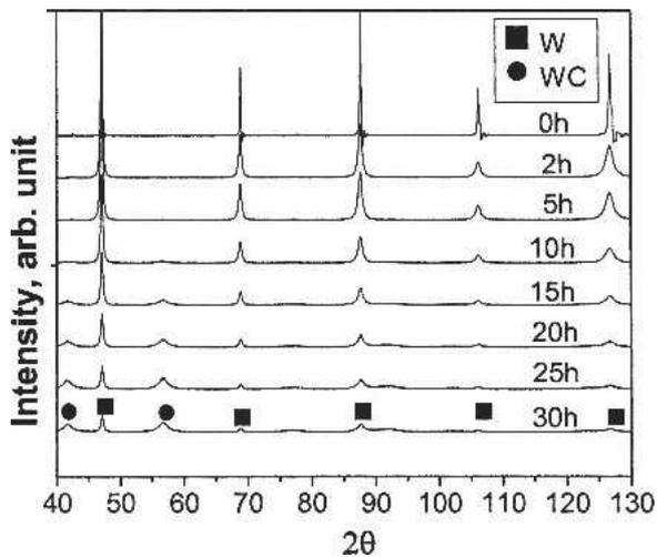
FIG. 2. XRD patterns of W powder as a function of MM time.
