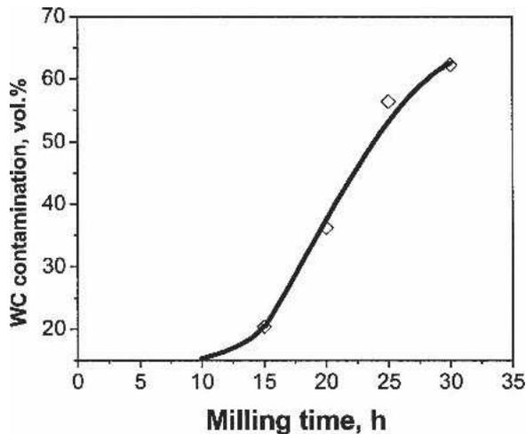
FIG. 6. Extent of WC contamination during MM of W up to 30 h.
