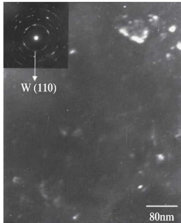
FIG. 4. Dark-field TEM image of W powder milled for 5 h revealing suitably oriented crystallites as bright regions. The electron diffraction pattern of this nanostructured powder in the inset displays the typical ring pattern of W.
