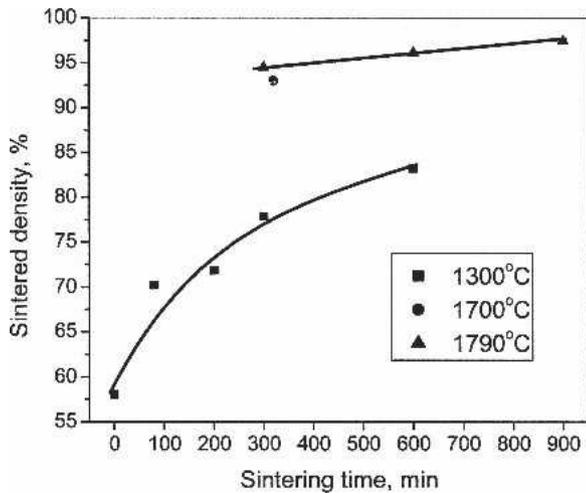
FIG. 8. Sinterability of W at 1300, 1700, and 1790 °C.
