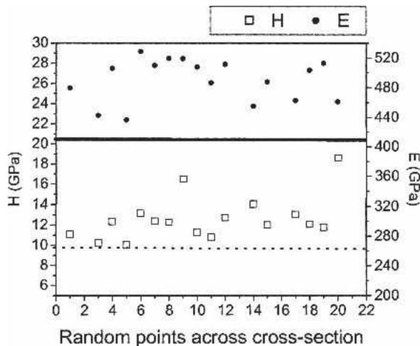
FIG. 10. Nanoindentation hardness (H) and elastic modulus (E) of W sintered at 1700 °C for 320 min. Corresponding values of H and E for microcrystalline W reported in the literature<sup>1–3</sup> are shown by dotted and solid bold lines, respectively.
