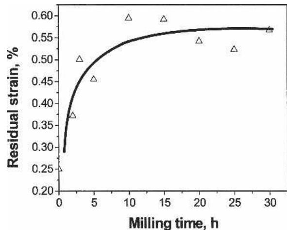
FIG. 5. Variation of the rms strain of W with milling time.
