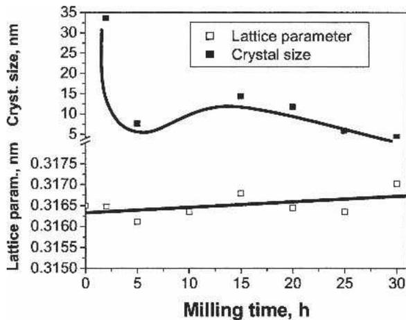
FIG. 3. Variations of crystal size and lattice parameter of W with milling time.
