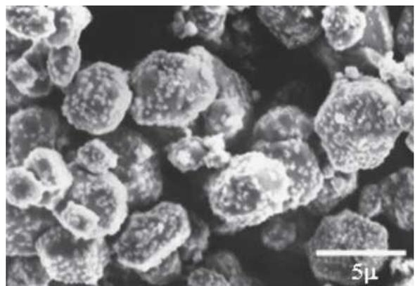
FIG. 1. SEM image of the as-received W powder.
