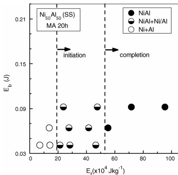
Fig. 10. Milling map for NiAl formation on MA of  $\text{Ni}_{50}\text{Al}_{50}$  with stainless steel media.
