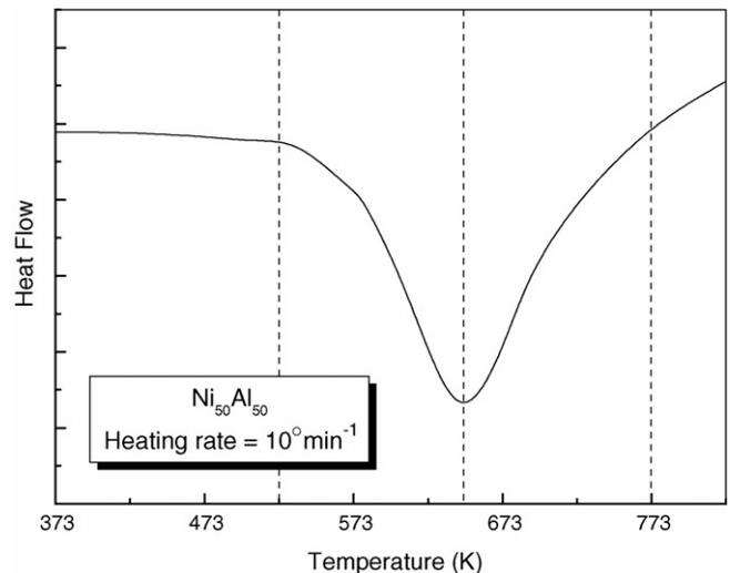
Fig. 5. DSC of NiAl mechanically alloyed for 20 h in tungsten carbide media from equiatomic Ni–Al blend at 300 rpm and ball-to-powder weight ratio of 10.
