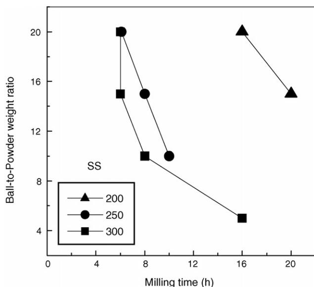
Fig. 6. Parametric phase diagram for NiAl formation during MA with stainless steel media.
