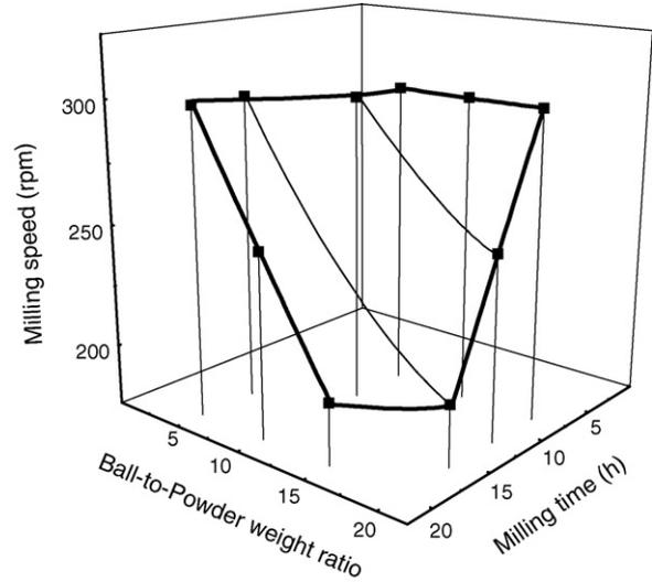
Fig. 4. 3-Dimensional parametric phase diagram with tungsten carbide media indicating the expansion of NiAl domain during MA.
