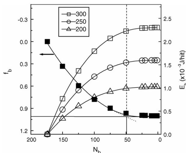
Fig. 1. Variation in shock frequency ( $f_b$ ) and ball energy ( $E_b$ ) with number of balls ( $N_b$ ).
