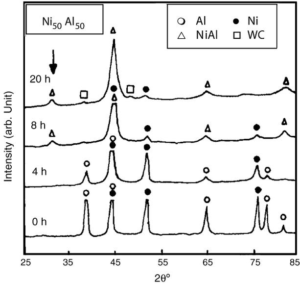
Fig. 2. XRD patterns showing the evolution of nanocrystalline NiAl during MA in  $\text{Ni}_{50}\text{Al}_{50}$  elemental blend milled in tungsten carbide media at 300 rpm and ball-to-powder weight ratio of 10. The NiAl superlattice reflection is shown by the arrow mark.
