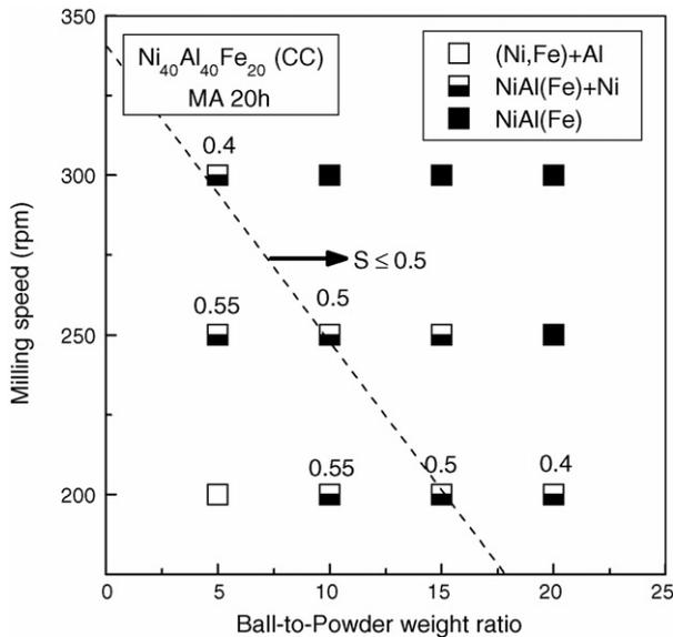
Fig. 8. Parametric phase diagram for NiAl(Fe) formation as well as change in long-range order parameter ( $S$ ) during MA of ternary blend of  $\text{Ni}_{40}\text{Al}_{40}\text{Fe}_{20}$  in tungsten carbide media.
