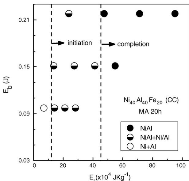
Fig. 11. Milling map for the formation of NiAl(Fe) on MA of  $\text{Ni}_{40}\text{Al}_{40}\text{Fe}_{20}$  with tungsten carbide media.
