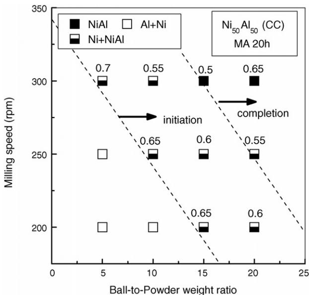
Fig. 3. Parametric phase diagram of NiAl prepared with tungsten carbide media after 20 h of MA. The numbers on the data points refer to the long-range order parameter.
