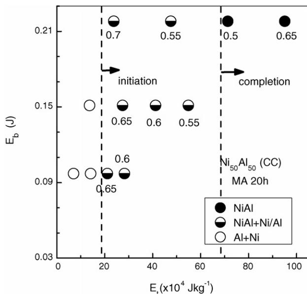
Fig. 9. Milling map for NiAl formation on MA of  $\text{Ni}_{50}\text{Al}_{50}$  with tungsten carbide media along with changes in long-range order parameter ( $S$ ) at various milling energies.
