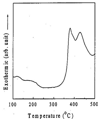
Fig. 7. DSC thermogram of the  $\text{Al}_{65}\text{Cu}_{20}\text{Nb}_{15}$  alloy measured in Ar atmosphere at  $20\text{ °C min}^{-1}$  heating rate following mechanical alloying in a planetary mill for 40 h showing overlapping double crystallization peaks approximately at 380 and 428 °C, respectively.
