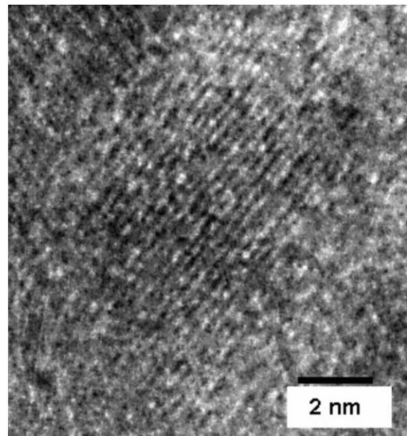
Fig. 5. High resolution TEM image of  $\text{Al}_{65}\text{Cu}_{20}\text{Nb}_{15}$  following mechanical alloying in a planetary mill for 20 h. Note that the microstructure is nanocrystalline with some intervening regions being amorphous with no well defined crystallinity or lattice fringes.
