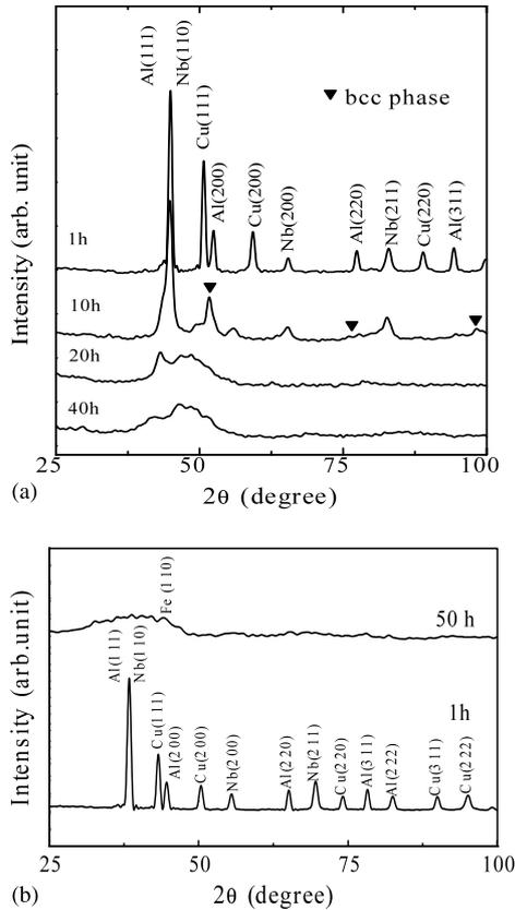
Fig. 3. XRD patterns showing phase evolution in the ternary  $\text{Al}_{65}\text{Cu}_{20}\text{Nb}_{15}$  alloy at different stages of mechanical alloying in (a) a planetary ball mill using WC vial and balls, and (b) a shaker mill using steel vial and balls. Note that the final milling product from both the mills is precisely identical (amorphous). XRD patterns of (a) and (b) were obtained using Co-K $\alpha$  and Cu-K $\alpha$  radiation, respectively.
