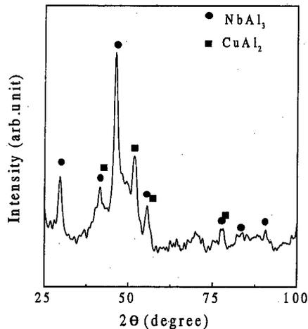
Fig. 8. XRD pattern of the ternary  $\text{Al}_{65}\text{Cu}_{20}\text{Nb}_{15}$  alloy following mechanical alloying in a planetary mill for 40 h and subsequent isothermal annealing at  $450^\circ\text{C}$  for 2 h in vacuum. Note that the annealed microstructure comprises nanocrystalline  $\text{NbAl}_3$  and  $\text{CuAl}_2$ .
