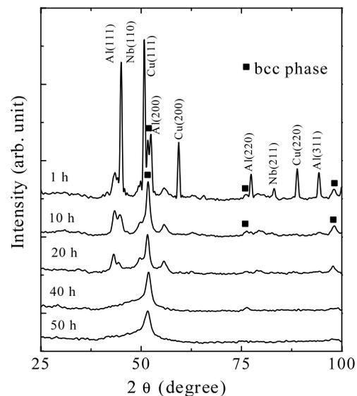
Fig. 2. XRD patterns showing the identity and sequence of phase evolution in the ternary Al<sub>65</sub>Cu<sub>30</sub>Nb<sub>5</sub> blend at different stages of mechanical alloying in a planetary mill up to 50 h. Note that the final milling product is a single phase disordered bcc solid solution.
