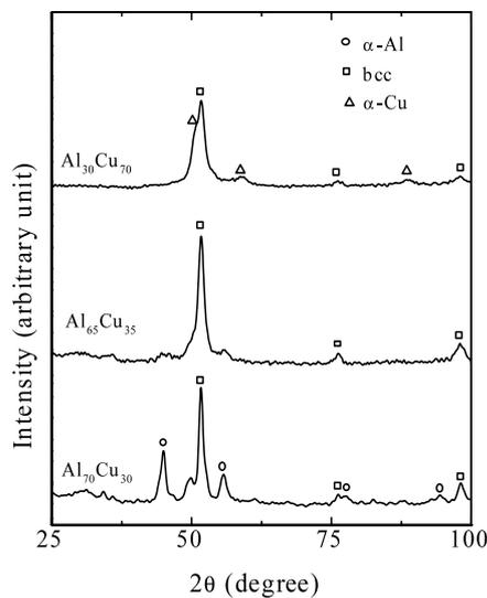
Fig. 1. XRD patterns of selected binary Al–Cu blends following isochronal mechanical alloying for 30 h in a planetary ball mill. Note that the milling product consists of two phases for the terminal compositions but a single phase nanocrystalline disordered bcc solid solution for the Al+35 at.% Cu blend.
