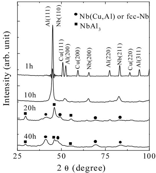
Fig. 4. XRD patterns showing phase evolution in the ternary  $\text{Al}_{65}\text{Cu}_{10}\text{Nb}_{25}$  alloy at different stages of mechanical alloying in a planetary mill. Note that the final milling product is a mixture of two nanocrystalline phases ( $\text{NbAl}_3$  and either  $\text{Nb}(\text{CuAl})$  or  $\text{fcc-Nb}$ ).
