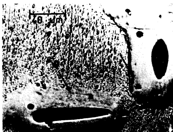
Fig. 1. The microstructure of Al–0.57%Si alloy displaying two dissolving silicon precipitates. The arrows indicate the silicon-enriched regions enveloping the precipitates and the mottled structure elsewhere is the precipitate-depleted matrix.
