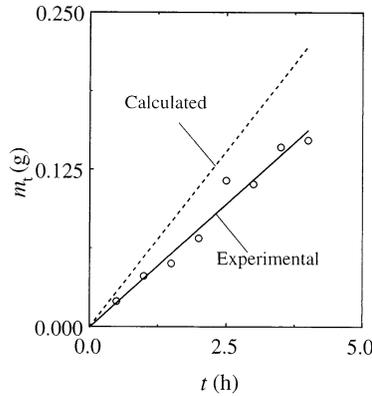
Figure 4. Variation of accumulated total mass ( $m_t$ ) of electrodeposited Cu and codeposited NbAl<sub>3</sub> with electrodeposition time ( $t$ ).
