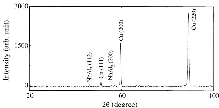
Figure 8. An XRD pattern of a sample surface following codeposition of NbAl<sub>3</sub> along with electrodeposition of Cu (from an 8 g/l CuSO<sub>4</sub> solution with a pH value of 3.5 and containing colloidal dispersion of 2 g/l of nanocrystalline NbAl<sub>3</sub> particles) on pure Cu cathode obtained using Co-K<sub>α</sub> radiation. The NbAl<sub>3</sub> peaks confirm the presence of these nanocrystalline aluminides on the codeposited surface.
