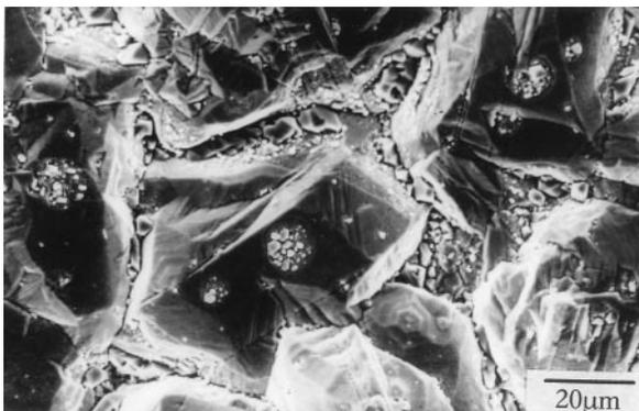
Figure 6. Distribution of codeposited NbAl<sub>3</sub> particles both along the grain boundaries as well as within the grain bodies of electrodeposited Cu on pure Cu substrate. Deposition condition was same as that in Fig. 5 except that,  $w = 4$  g/l.
