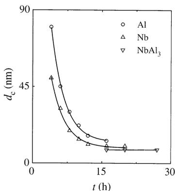
Figure 2. Variation of crystallite size ( $d_c$ ) of Nb, Al and NbAl<sub>3</sub> (formed by mechanical alloying) as a function of cumulative milling time ( $t$ ).
