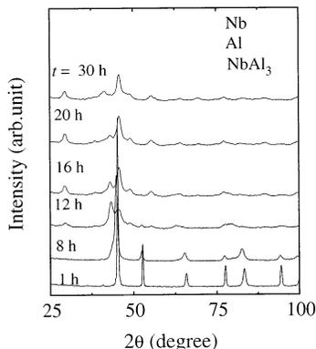
Figure 1. A series of XRD patterns obtained from a powder blend of Nb<sub>25</sub>Al<sub>75</sub> following mechanical alloying for different periods of cumulative milling time ( $t$ ).
