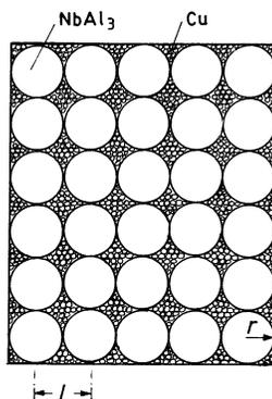
Figure 3. A schematic representation of the assumed distribution of codeposited nanocrystalline NbAl<sub>3</sub> particles in the electrodeposited Cu matrix.
