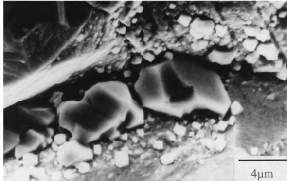
Figure 7. Magnified view of Fig. 6 to show that NbAl<sub>3</sub> particles are deposited with a varying size distribution from nanocrystalline or submicron size (within grain bodies) to occasionally coarse/agglomerated form (along grain boundaries).
