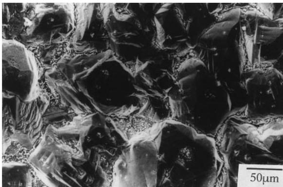
Figure 5. An SEM micrograph showing the codeposited ultrafine NbAl<sub>3</sub> particles along the grain boundaries of electrodeposited Cu. Codeposition was carried out with electrodeposition from a CuSO<sub>4</sub> solution (8 g/l and 3.5 pH) containing  $w = 1$  of colloiddally dispersed NbAl<sub>3</sub> particles at 4 V for  $t = 200$  min.
