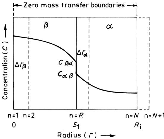
Fig. 4. Modified representation of the finite difference nomenclature presented in Fig. 3 following the consumption of liquid.
