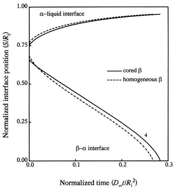
Fig. 11. Effect of coring in  $\beta$  on the kinetics of peritectic transformation for an alloy of composition  $C_0 = 0.23$  in Fig. 7(b) at  $T_1$ .
