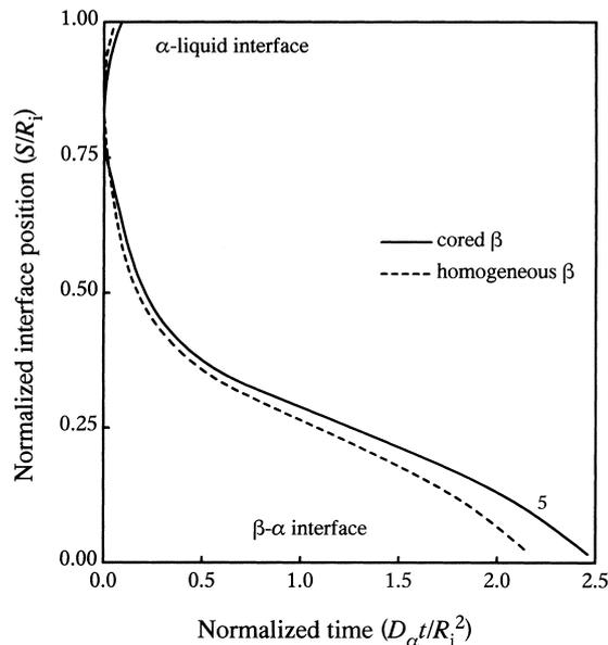
Fig. 12. Influence of solute segregation in  $\beta$  on the kinetics of peritectic and  $\beta$ - $\alpha$  transformation following liquid consumption for an alloy of peritectic composition in Fig. 7(b) at  $T_1$ .
