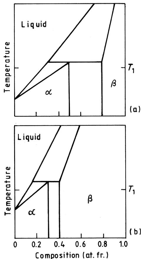
Fig. 7. (a, b) Schematic peritectic phase diagrams utilized to calculate the effect of coring in the solids on the peritectic transformation kinetics.
