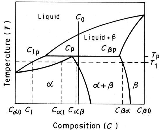
Fig. 1. A schematic binary peritectic phase diagram defining the concentration terms used in the model.
