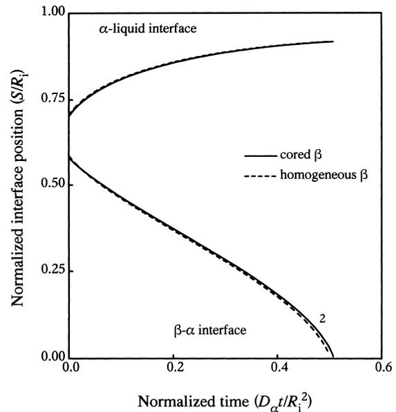
Fig. 9. Influence of concentration profile in  $\beta$  on the kinetics of peritectic transformation illustrated in Fig. 7(a) for an alloy composition  $C_0 = 0.45$  at  $T_1$ .
