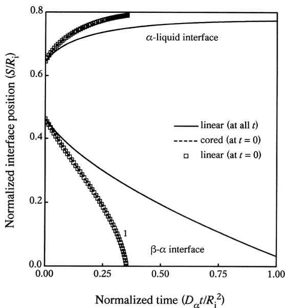
Fig. 8. Effect of concentration profile in  $\alpha$  on the kinetics of the peritectic transformation shown in Fig. 7(a) at  $T_1$ .
