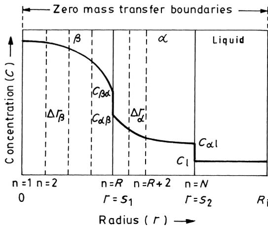
Fig. 3. Schematic concentration–distance profiles illustrating the finite difference nomenclature adopted for the spherical cell in Fig. 2.
