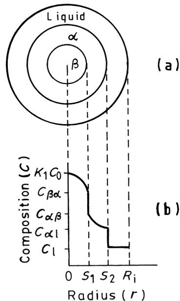
Fig. 2. (a) Schematic representation of the idealized peritectic transformation cell and, (b) the concentration-distance profiles in it during isothermal transformation in an alloy of composition  $C_0$  of Fig. 1 at  $T_1$ .  $K_1$  is the equilibrium solute distribution coefficient between  $\beta$  and liquid.
