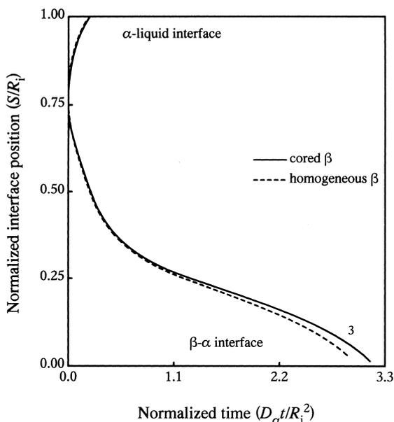
Fig. 10. Kinetics of peritectic and  $\beta$ - $\alpha$  transformation following liquid consumption in the presence of cored or homogeneous  $\beta$ -phase for an alloy of peritectic composition in Fig. 7(a) at  $T_1$ .
