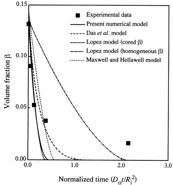
Fig. 5. Volume fraction of the  $\beta$ -phase as a function of normalized time ( $D_\alpha t/R_i^2$ ) for isothermal peritectic transformation in a Cd-5 at.% Ag alloy at 608 K.
