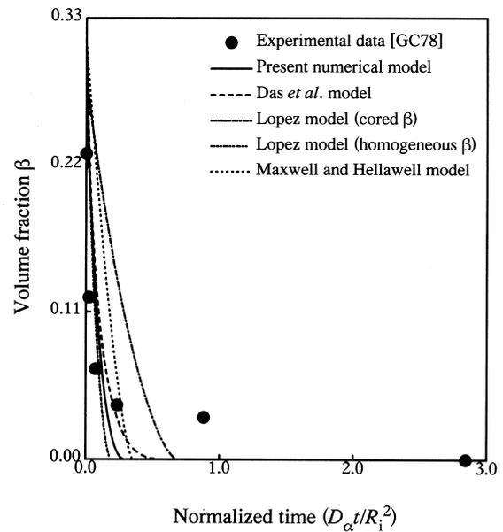
Fig. 6. Kinetics of peritectic transformation in a Pb-33.3 wt% Bi alloy at 443 K.
