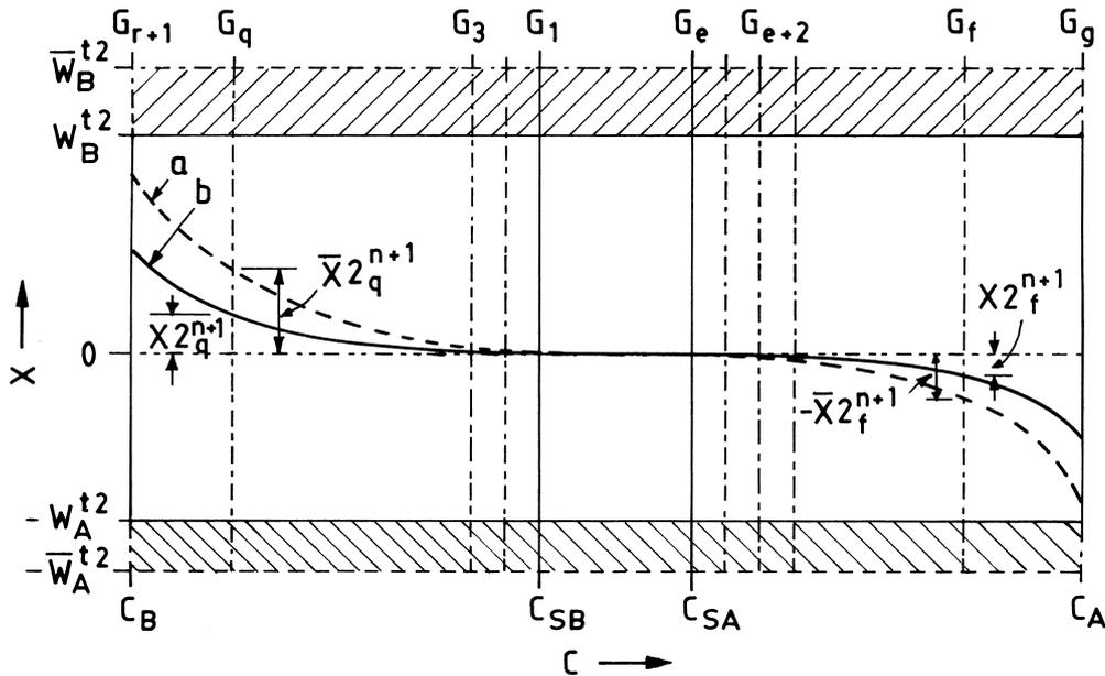
Fig. 5. Schematic distance ( $X$ )-concentration ( $C$ ) profiles at  $t_2$ . Curve-a and curve-b represent the profiles after considering interdiffusion alone, and its modification by incorporating deformation, respectively.
