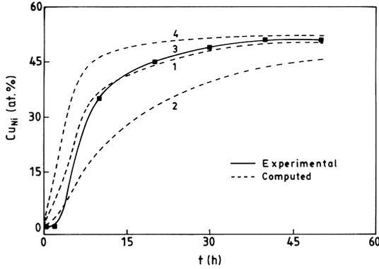
Fig. 8. Variation of Ni-content in Cu-solid solution ( $\text{Cu}_{\text{Ni}}$ ) with milling time ( $t$ ) for  $\text{Cu}_{20}\text{Ni}_{80}$  milled at 300 rpm. Curve-1 represents the experimentally determined data. Curve-2, curve-3 and curve-4 are computed data obtained for  $D = D_v$  (at  $T = 745$  K),  $D = D_v$  ( $T_{\text{eff}} = 785$  K) and  $D = D_v$  ( $T = 825$  K), respectively.
