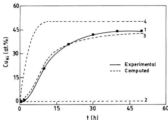
Fig. 7. Variation of Ni-content in Cu-solid solution (Cu<sub>Ni</sub>) with milling time ( $t$ ) for Cu<sub>50</sub>Ni<sub>50</sub> blend milled at 300 rpm. Curve-1 represents the experimentally determined data. Curve-2, curve-3 and curve-4 are computed data obtained for  $D = D_v$  (at  $T = 553 \text{ K}$ ),  $D = D_v$  ( $T_{\text{eff}} = 775 \text{ K}$ ) and  $D = D_{\text{gb}}$  ( $T = 373 \text{ K}$ ), respectively.
