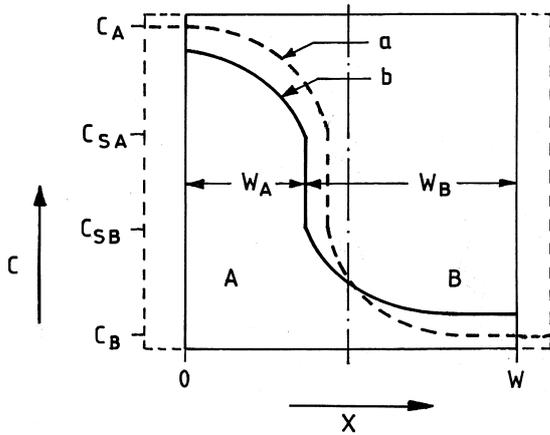
Fig. 4. Effect of time on *iso*-concentration contour representing the combined contributions of diffusion and deformation. Note that curve-a and curve-b correspond to time  $t'$  and  $t'' (> t')$ , respectively.
