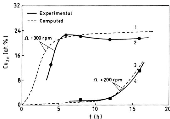
Fig. 9. Variation of Zn-content in Cu-solid solution ( $\text{Cu}_{\text{Zn}}$ ) with milling time ( $t$ ) for the  $\text{Cu}_{70}\text{Zn}_{30}$  blend milled at 300 and 200 rpm. Curve-1 and curve-3 are computed for  $D = D_{\text{v}}$  at  $T = 520$  and 505 K, respectively.
