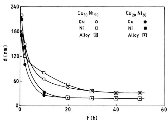
Fig. 6. Experimental data on variation of crystallite size ( $d$ ) with milling time ( $t$ ) of Cu and Ni in the Cu<sub>20</sub>Ni<sub>80</sub> and Cu<sub>50</sub>Ni<sub>50</sub> blends.
