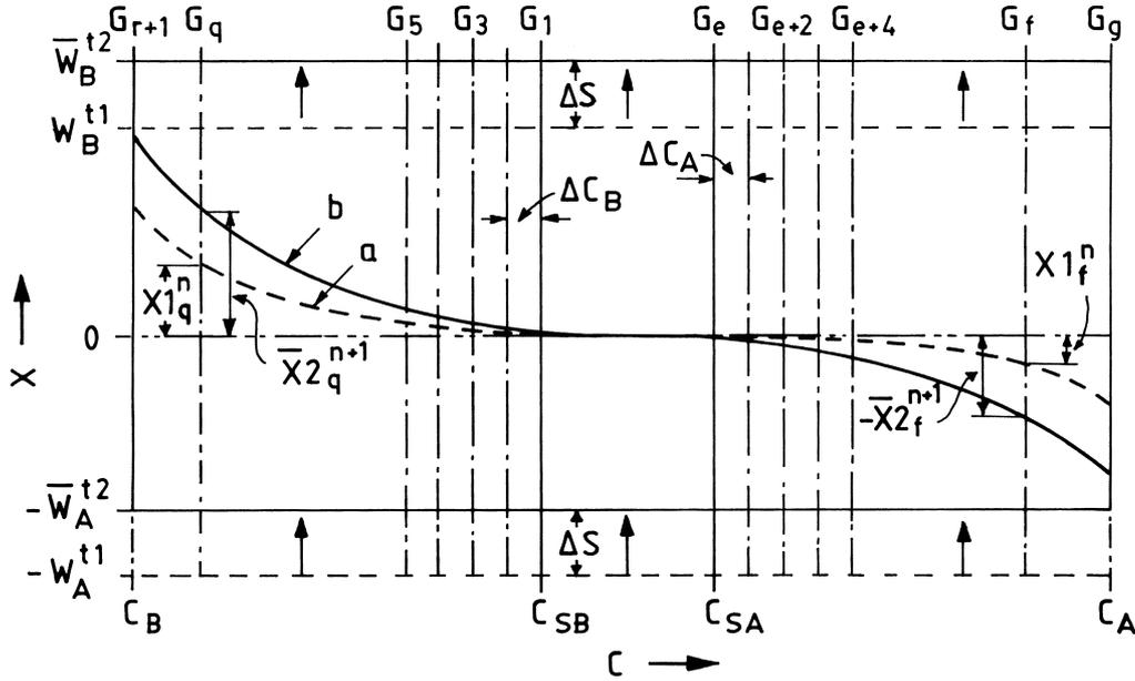
Fig. 3. Illustration of the finite difference terminology used in the MICCM model. Curve-a and curve-b represent the schematic plots of distance ( $X$ )-concentration ( $C$ ) profile at time  $t_1$  and following interdiffusion at  $t_2$ , respectively.
