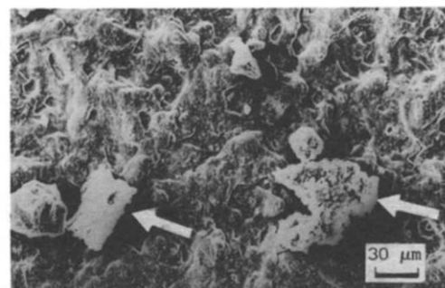
Fig.4: Particulate phases (shown by arrowhead) appearing in the microstructure after eight laser pulses.
