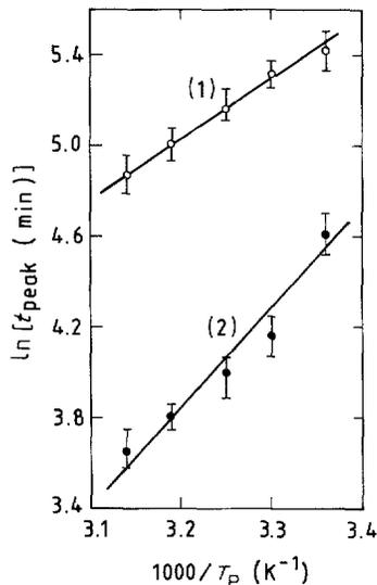
Figure 2 Plot of  $\ln t_{\text{peak}}$  against  $1000/T_p$ . Curve 1 is obtained for  $T_M = T_p$  while for Curve 2  $T_M = -196^\circ\text{C}$ .
