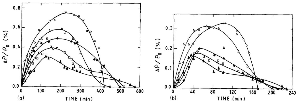
Figure 1 Fractional change in resistivity,  $\Delta\rho/\rho_0$ , with time  $t$ , measured at (a)  $T_M = T_p$  and (b)  $T_M = -196^\circ\text{C}$ . The precipitation temperatures ( $T_p$ ) are (○)  $25^\circ\text{C}$ , (Δ)  $30^\circ\text{C}$ , (●)  $35^\circ\text{C}$ , (□)  $40^\circ\text{C}$  and (▲)  $45^\circ\text{C}$ .
