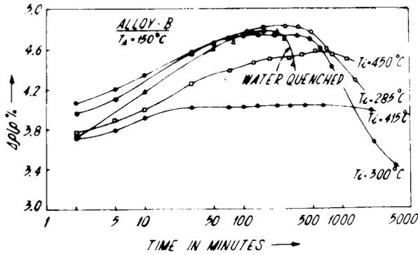
Fig. 3. Variation of resistivity of alloy B with time at  $150^\circ\text{C}$ , following pretreatments as indicated.
