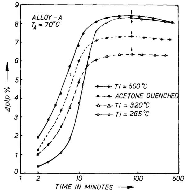
Fig. 1. Variation of resistivity of alloy A with time at 70°C, following pretreatments as indicated; the arrows indicate the resistivity-peak positions.
