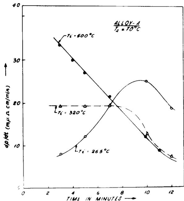
Fig. 5. Rate of increase in resistivity during zone formation as a function of time.
