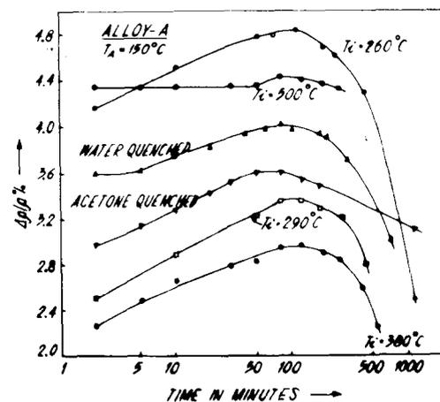
Fig. 2. Variation of resistivity of alloy A with time at 150°C, following pretreatments as indicated.
