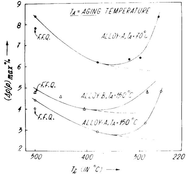
Fig. 4. Variation of resistivity maxima of isothermal aging with the temperature of quench interruption; F. F. Q. corresponds to aging following a free-fall-quench into water from  $500^\circ\text{C}$ .
