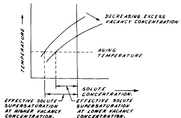
Fig. 6. Schematic illustration of the change in solute supersaturation with excess-vacancy concentration.
