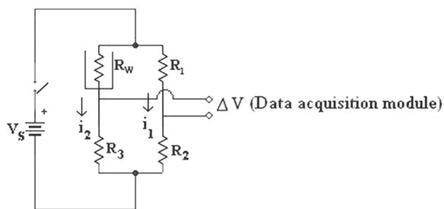
**Fig. 1.** Schematic diagram of transient hot-wire set up used in the present experiments to measure the thermal conductivity of nanofluids.
