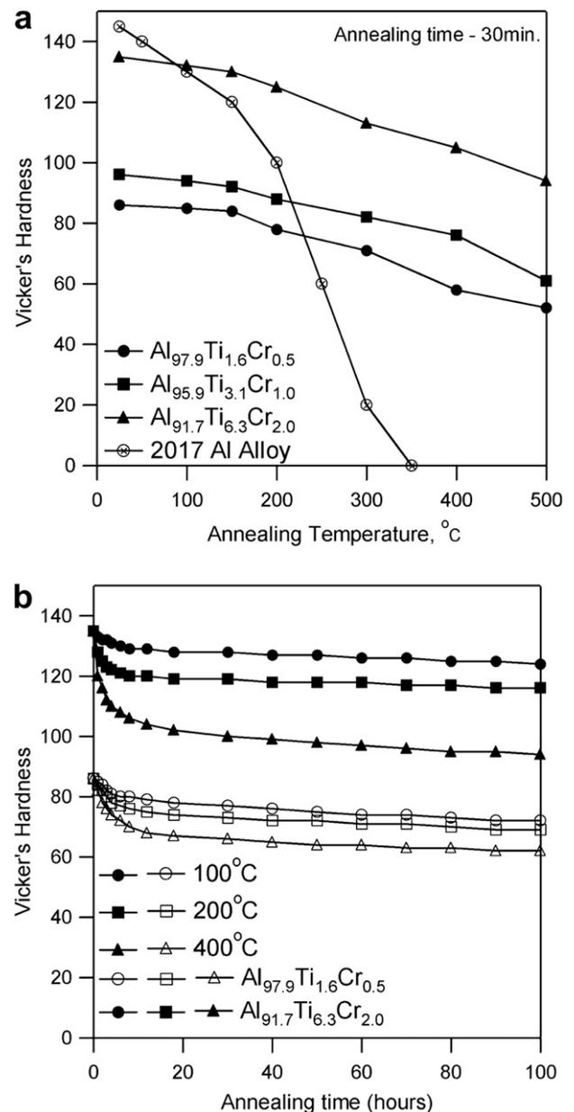
**Fig. 6.** Variation of Vickers hardness of melt spun ternary Al–1.6Ti–0.5Cr, Al–6.3Ti–2.0Cr alloys with (a) temperature and comparison with conventional 2017 Al alloy, and (b) holding time at temperature 100, 200 and 400 °C.
