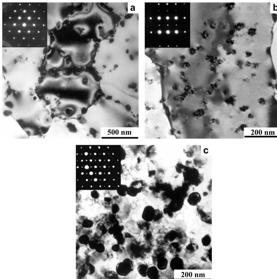
Fig. 4. Bright field TEM images of (a) Al-1.6Ti-0.5Cr, (b) Al-3.2Ti-1.0Cr and (c) Al-6.3Ti-2.0Cr alloys melt spun at 30 m/s. Insets are the SAD patterns of the  $L_{12}$ - $Al_3Ti$  particles.
