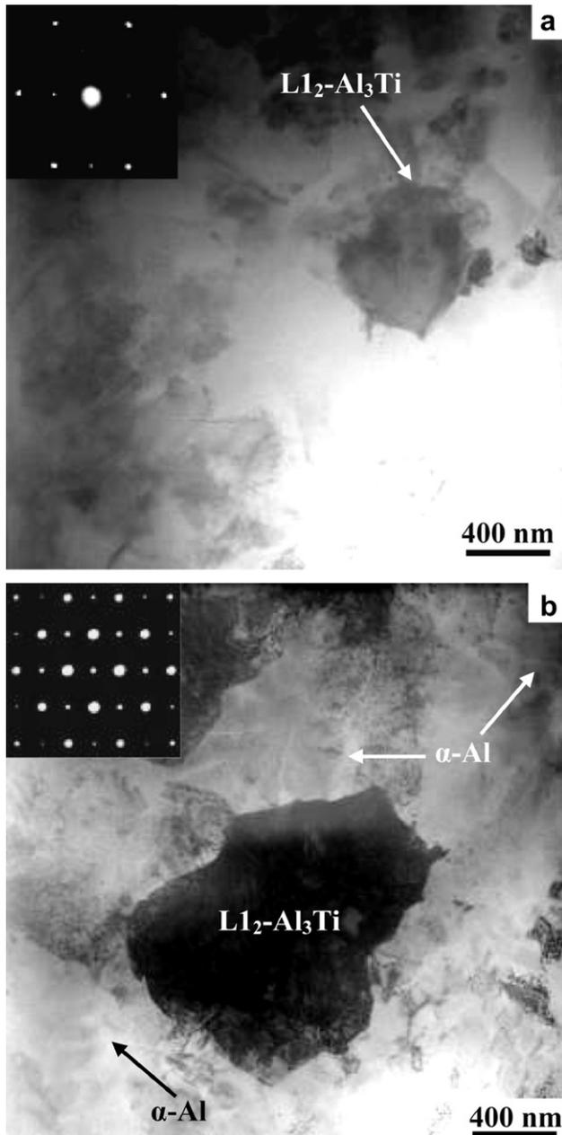
**Fig. 2.** Bright field images of (a) Al-5Ti and (b) Al-15Ti alloys melt spun at 40 m/s wheel velocity. Insets are the selected area diffraction patterns from the  $L_{12}$ - $Al_3Ti$  particles in respective alloys.
