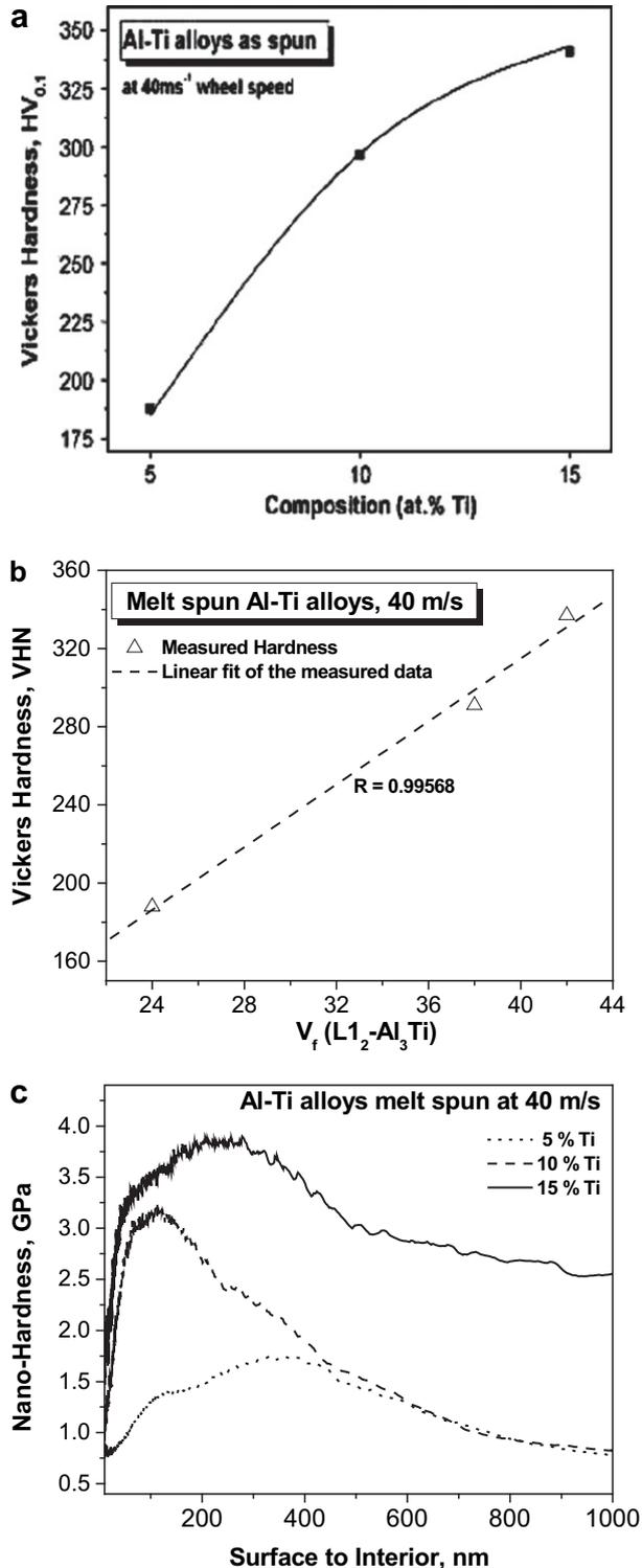
**Fig. 5.** Hardness of Al–Ti alloys melt spun at 40 m/s wheel velocity. (a) Variation of Vickers hardness with Ti content, (b) Variation of Vickers hardness with volume fraction of  $L1_2$ - $Al_3Ti$  phase in the nanocomposites, and (c) Hardness variation in nanoindentation studies with depth from the surface.
