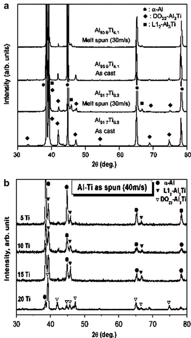
Fig. 1. XRD patterns of (a) as-cast and melt spun (30 m/s) Al–4.1Ti and Al–8.3Ti alloys and (b)  $Al_{100-x}Ti_x$ ,  $x = 5, 10, 15$  and 20, alloys melt spun at higher cooling rate (40 m/s).
