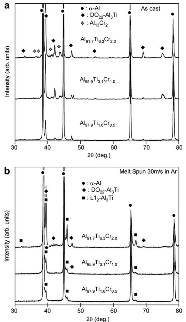
**Fig. 3.** XRD patterns of (a) as-cast and (b) melt spun (30 m/s) ternary Al-1.6Ti-0.5Cr, Al-3.2Ti-1.0Cr and Al-6.3Ti-2.0Cr alloys.
