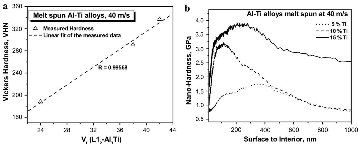
**Fig. 2** Hardness of Al–Ti alloys melt spun at 40 m/s wheel velocity: **a** Vickers hardness as a function of volume fraction of  $L1_2$ - $Al_3Ti$ ; **b** variation of nano-hardness with depth from the surface of the specimen [10, 16]
