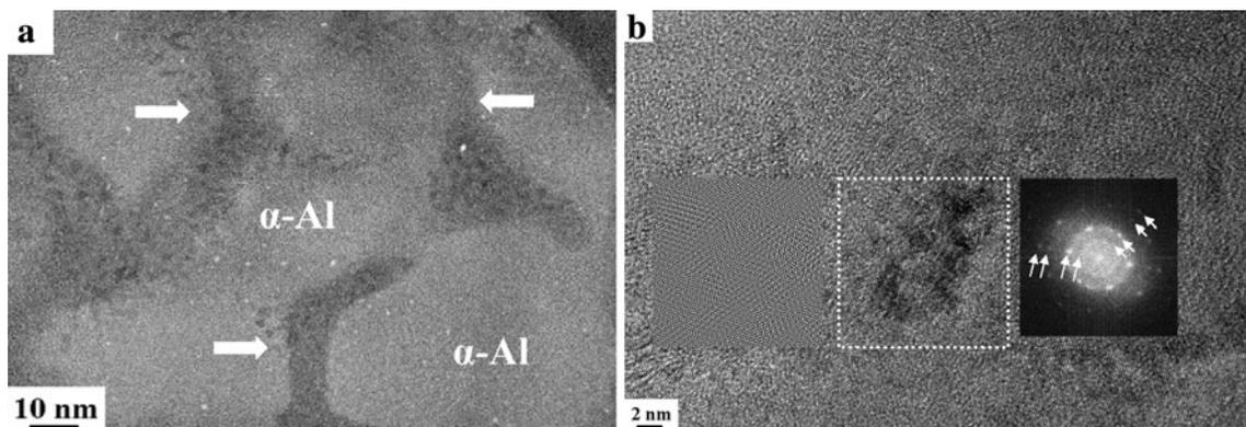
**Fig. 3** HRTEM images of Al-5Fe alloy melt spun at 40 m/s: **a** low-magnification image showing nano-cellular structure with distribution of dark NQ particles, **b** high magnification image depicting NQ phase: inset FFT-SAED pattern on *right* in **b** was obtained from the *square marked region* revealing the 3-fold symmetry pattern, and the reverse FFT image is shown on *left* side [15, 16]
