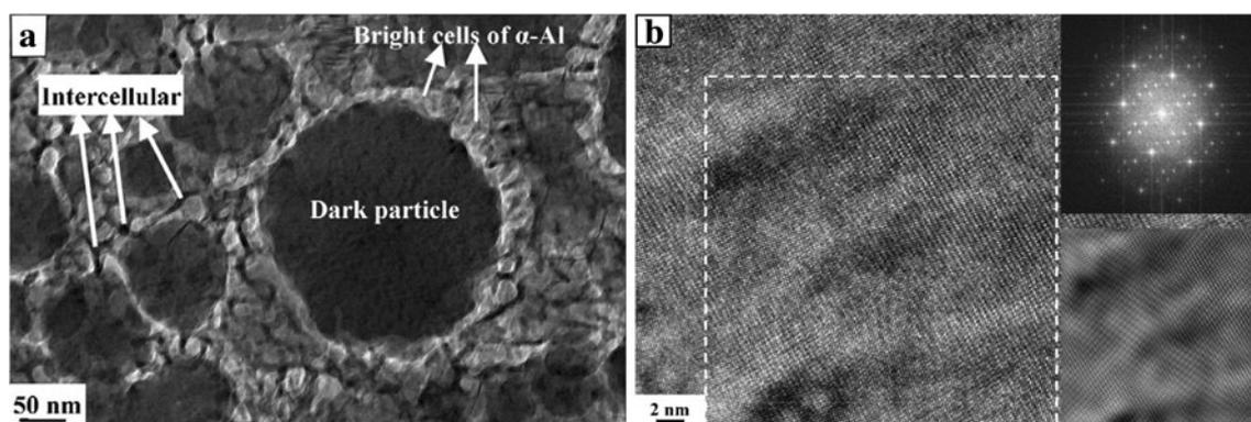
**Fig. 4** HRTEM images of Al-10Fe alloy melt spun at 40 m/s: **a** showing microstructure with NQ nodules embedded in cellular matrix of  $\alpha$ -Al with intercellular NQ regions, **b** illustrating NQ phase. 2-fold symmetry in the FFT-SAD pattern (*top-right* inset in **b**) and inverse FFT from the FFT-SAD pattern (*bottom-right* inset in **b**) are also displayed [15, 16]
