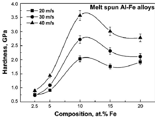
**Fig. 5** Variation of microhardness as a function of Fe content in Al–Fe alloys melt spun at different wheel speeds [15, 16]
